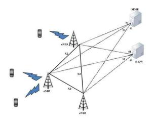
Fig. 1 LTE-A network architecture
