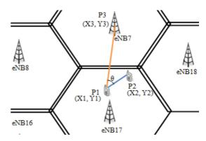
Fig. 3 Angle calculation for candidate eNBs
