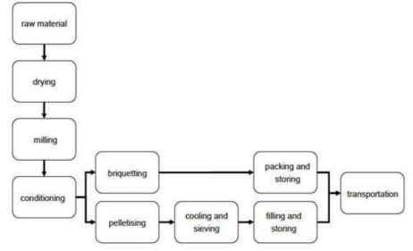
Fig. 3 Process of pellet production and briquette
