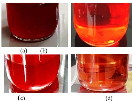
Fig. 6 (a) Retentate and (b) permeate of fermented beetroot at TMP 2 bar, (c) retentate and (d) permeate of fermented beetroot at TMP 6 bar passed through CF-MF at room temperature and flow rate  $\sim 7.5$  L/min. for 35 minutes.
