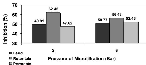
Fig. 7 Relationship of type of fermented beetroot and TMP on inhibition ability via CF-MF at flow rate  $\sim 7.5$  L/min. for 35 minutes.
