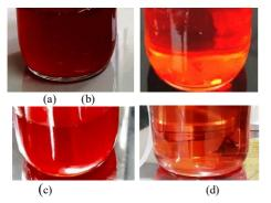
Fig. 6 (a) Retentate and (b) permeate of fermented beetroot at TMP 2 bar, (c) retentate and (d) permeate of fermented beetroot at TMP 6 bar passed through CF-MF at room temperature and flow rate  $\sim$ 7.5 L/min. for 35 minutes.
