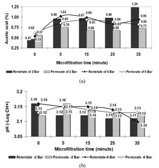
Fig. 4 Relationship of TMP and time on (a) acetic acid and (b) pH in fermented beetroot by CF-MF.
