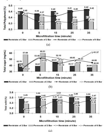
Fig. 5 Relationship of TMP and time on (a) total polyphenols, (b) total sugars, and (c) total solids in fermented beetroot by CF-MF.
