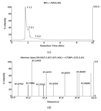
Fig. 9 (a) Chromatogram of gallic acid and (b) mass spectra of gallic acid at room temperature, flow rate  $\sim$ 7.5 L/min. and TMP 6 bar for 35 minutes, (c) chromatogram of acetic acid and (d) mass spectra of acetic acid at room temperature, flow rate  $\sim$ 7.5 L/min. and TMP 2 bar for 35 minutes
