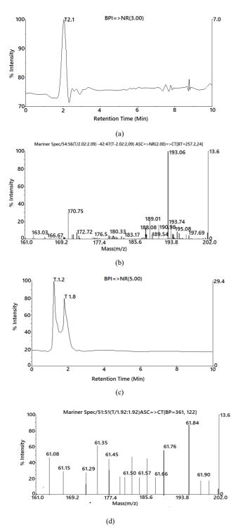
Fig. 8 (a) Chromatogram of standard gallic acid and (b) mass spectra of standard gallic acid ( $M+Na^+$ ), (c) chromatogram of standard acetic acid and (d) mass spectra of standard acetic acid ( $M^+$ ).
