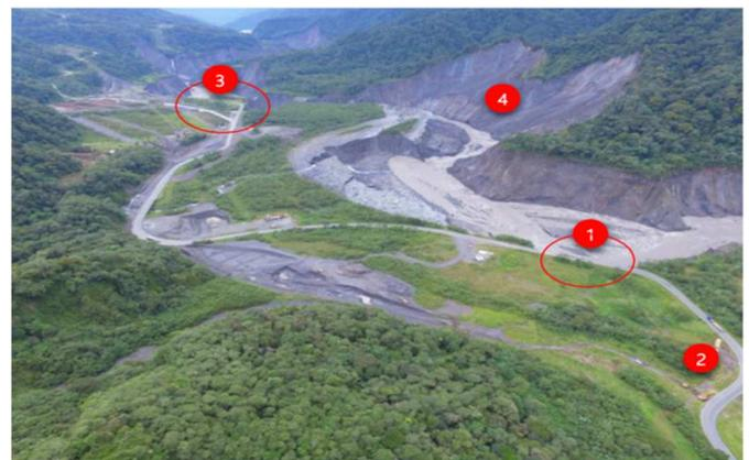
Fig. 3 Road situation due to the erosion of the river - road from Baeza to Lago Agrio. Hereby, from 1 to 4 are indicated the Chronological events in the river morphology: 1, Track loss at km 66 (22/08/2020); 2, Provisional variant for km 66; 3, Cracking of the track at the Bridge over the River Montana (04/06/2020) Track variation over the River Montana; 4, Large-scale landslide which partially dammed the Coca River. (20/07/2020)
