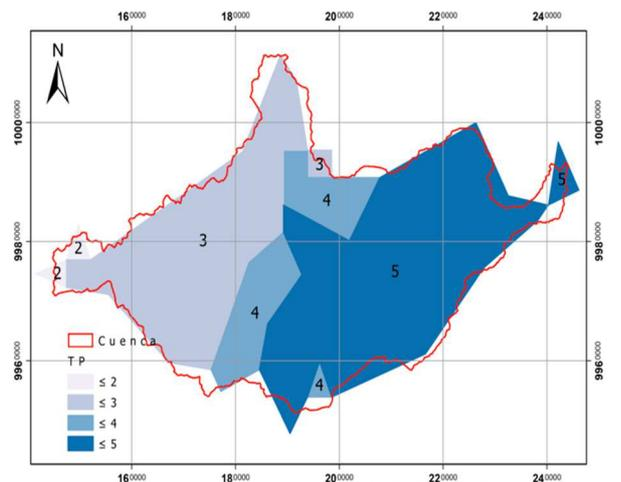
Fig. 7 This figure represents the intensity of rains (Tp) presents factors of 2 low in the 10 years the precipitation 51 to 91 mm, 3 medium presents precipitation 91-130 mm, high 131 to 175 mm and 5 very high, the precipitation is greater than 175 mm of rain in the last 10 years
