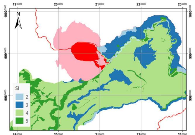
Fig. 5 The lithology represented in this figure presents a factor of 2 moderate classification, table formation, 3 medium, metamorphic rocks, 4 high volcanic deposits (lahars) and 5 very high that are slope deposits (colluvial)
