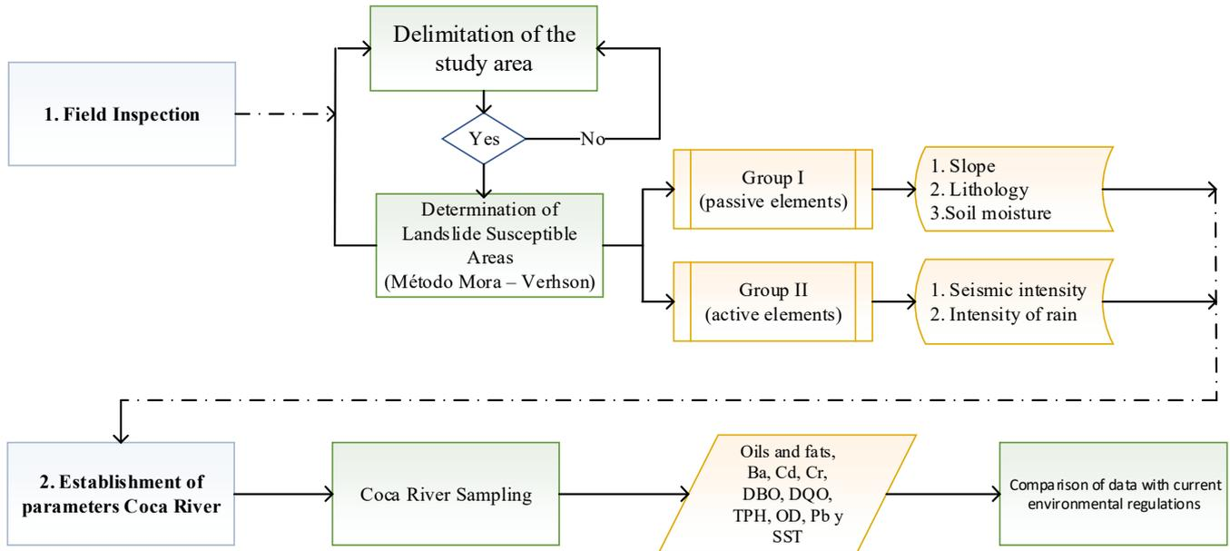
Fig. 2 Flow diagram which determines the areas susceptible to landslides in the Quijos - Coca River basin and environmental risk from the oil spill due to the SOTE and OCP rupture
