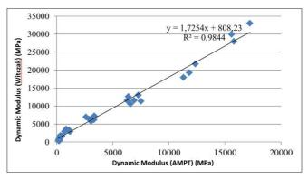
Fig. 3 Dynamic Modulus of Each Mixture Comparison
