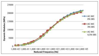
Fig. 2 Relationship between Dynamic Modulus and Reduced Frequency
