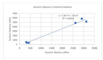
Fig. 5 Dynamic Modulus and Resilient Modulus Correlation
