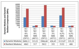
Fig. 4 Dynamic Modulus and Resilient Modulus Comparison
