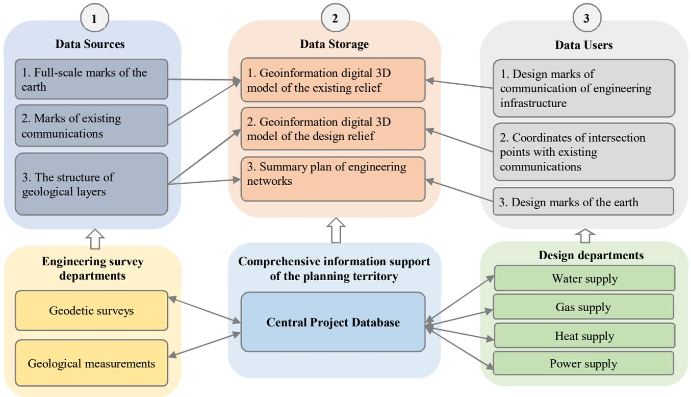
Fig. 4 BIM-structure of Central Project Database
