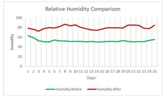
Fig. 7 Comparison between Smart Greenhouse Relative Humidity and Outside Greenhouse Relative Humidity
