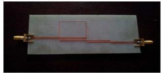
Fig. 11 Fabricated photo of the the first topology base on the base cell with second coupled-line
