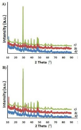
Fig. 3 XRD Chitosan CC Spectra. A). Deacetylation Long heating 60 minutes. B). Deacetylation Old Heating 120 minutes. a) 5% NaOH, b) 10% NaOH, c) 15% NaOH
