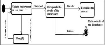
Fig. 6 Activity diagram of disturbance detection
