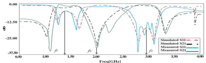
Fig. 8 Simulated and measured S11 and S21 results
