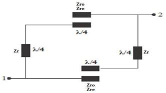
Fig.1 Dual-band bandpass filter topology
