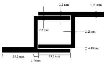
Fig. 3 Dimensions of the optimised dual-band bandpass filter
