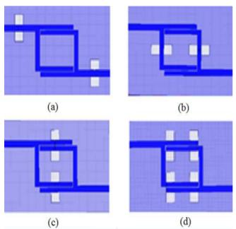
Fig. 6 DGS locations in the ground plane of the filter (a) feed lines (b) quarter wavelength lines (c) centre of parallel-coupled lines (d) edges of parallel-coupled lines
