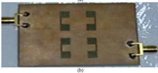
Fig. 11 Etched DGSs on dual-bandpass filter ground planes (a) one pair and (b) two pairs of DGSs  $\,$
