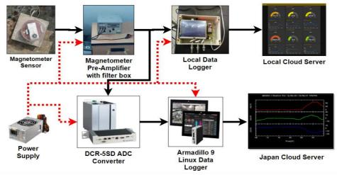
Fig. 6 The flow diagram of parallel data logger installation for MAGDAS at USM Pulau Pinang
