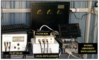
Fig. 7 The Installation of MAGDAS II YU-8T Magnetometer.
