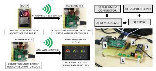
Fig. 5 The developed data logger used for MAGDAS installation.
