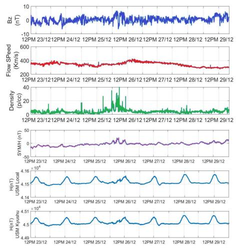
Fig. 12 The value of interplanetary Magnetic field, Bz, Flow Speed, Density of solar wind, SYM/H (nT), Local H(nT), and Kyushu H(nT) from the data logger.
