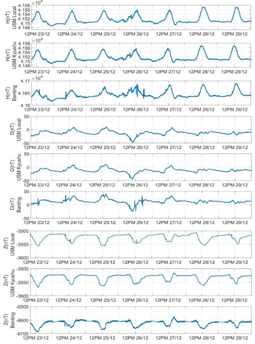
Fig. 10 The H, D and Z(nT) component magnetic field comparison between Local, Kyushu and banting data logger
