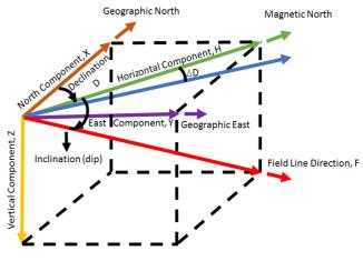
Fig. 3 The direction of magnetic field strength parameters
