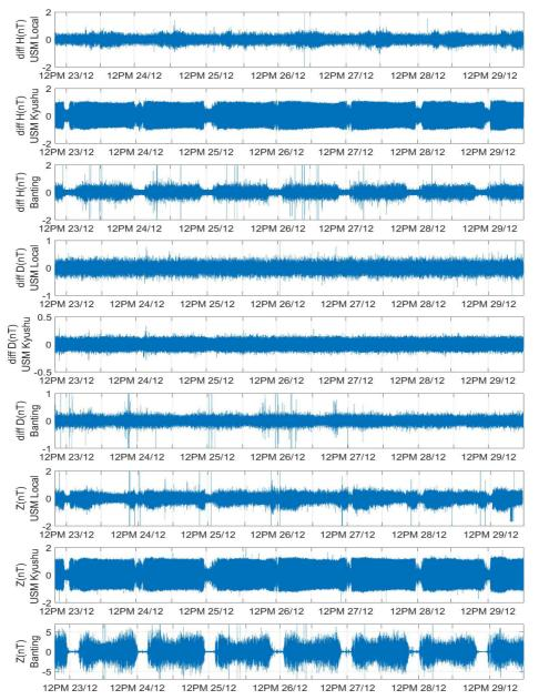
Fig. 11 The artificial noise from H, D and Z(nT) of Local, Kyushu and banting data logger
