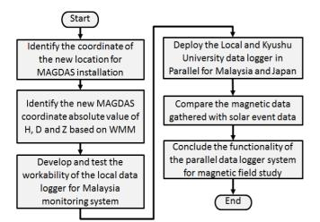
Fig. 2 Flow Diagram of the Method involved for MAGDAS installation
