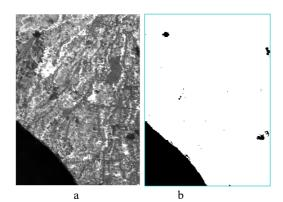
Fig. 8 Landsat 8 image results from the band ratio 5/3 (a) and after masking (b)
