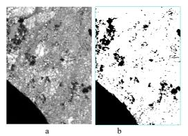
Fig. 6 Landsat 8 image before masking (a) and after masking (b) with threshold suppressors in band  $6\,$
