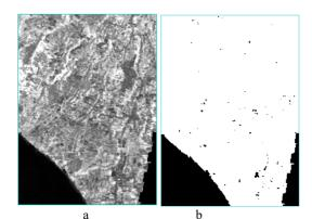
Fig. 7 Landsat 7 image results from the band ratio 4/2 (a) and after masking (b)
