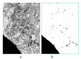
Fig. 5 Landsat 7 image before masking (a) and after masking (b) with threshold suppressors in band 5  $\,$
