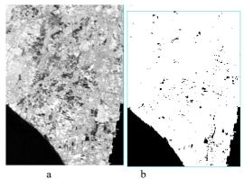
Fig. 9 Landsat 7 image results from band ratio 5/2 (a) and after masking (b)
