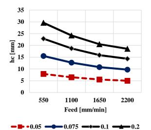
Fig. 8 hc values with S = 6000 rpm
