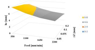
Fig. 9 The relationship diagram between hc with  $\Delta Z$  and F in S = 6000 rpm mode
