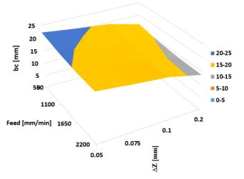
Fig. 7 Relationship diagram between bc with  $\Delta Z$  and F in S = 6000 rpm mode
