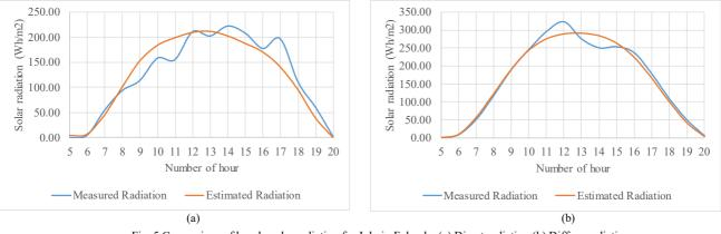
Fig. 5 Comparison of hourly solar radiation for July in Fukuoka (a) Direct radiation (b) Diffuse radiation
