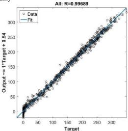
Fig. 3 Regression line of the ANN training for diffuse solar radiation estimation
