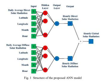
The target output was the average solar radiation for each hour, between Japan's earliest sunrise (5 AM) and the latest sunset (8 PM). The training data were the average hourly solar radiation measurements from three years (January 2016 through December 2018) in five locations, resulting in 960 samples for each data parameter.
