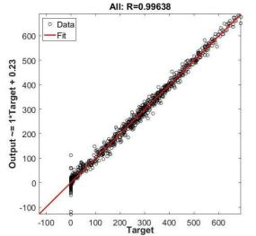
Fig. 2 Regression line of the ANN training for direct solar radiation estimation
