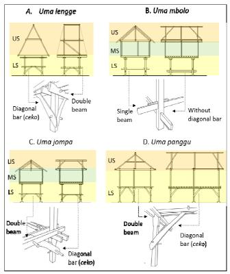
Fig. 5 Sections of *uma lengge* (A), *uma mbolo* (B), *uma jompa* (C), and *uma panggu* (D), which has some level: lower structure (LS), middle structure (MS), and upper structure (US), and also the comparison of their stilt structure.
