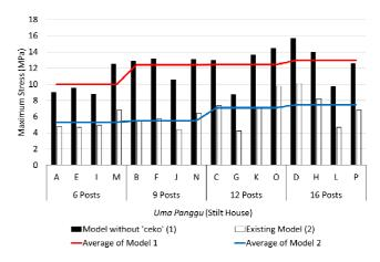
Fig. 9 Comparison of the maximum stress (MPa) between the models without diagonal bars (*ceko*) and existing models in each type of stage house (*uma panggu*)
