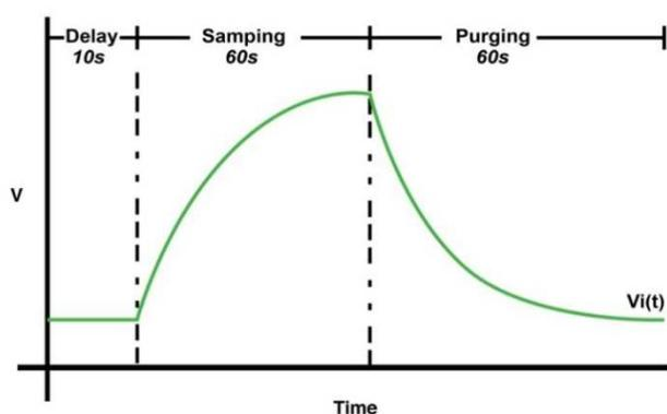
Fig. 2 Typical of response of a gas sensor to a sample. Time configuration setting in this study, for delay, sampling and purging were 10 s, 60 s, and 60 s, respectively.
