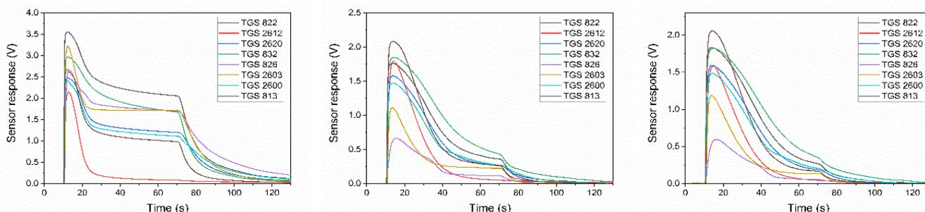
Fig. 4 Examples of the response on sensor array from raw data of measurement. Neutral (left), *E. coli* (middle), and *S. Typhimurium* (right).
