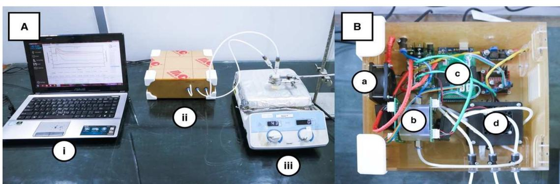
Fig. 1 A. A lab-made electronic-nose device. i: a computer equipped with chemometric tools, ii: the main part of e-nose, and iii: sample on the hot plate; and B. Part of e-nose device. a: power supply, b: sensor chamber, c: DAQ and controller, and d: sampling system
