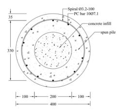
Fig. 3 Cross-section and reinforcement detail of specimens
