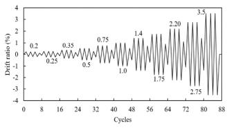
Fig. 6 The Sequence of drift ratio according to ACI 347-1-05 [15]
