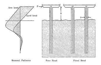
Fig. 2 Moment patterns in free and fixed-head piles [3]
