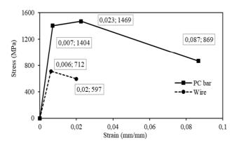
Fig. 4 Tensile stress-strain relationship of PC bar and spiral reinforcement
