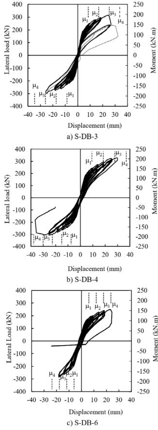
Fig. 8 The hysteresis load-displacement of the spun pile with concrete infill under 784 kN (0.16fc'Ag) of axial load
