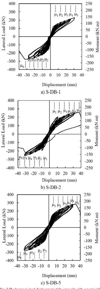
Fig. 7 The hysteresis load-displacement of the spun pile with concrete infill under 392 kN (0.08fc'Ag) of axial load
