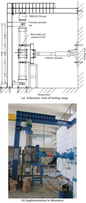
Fig. 5 Test setup of specimen and loading system for cyclic flexural with axial load testing
