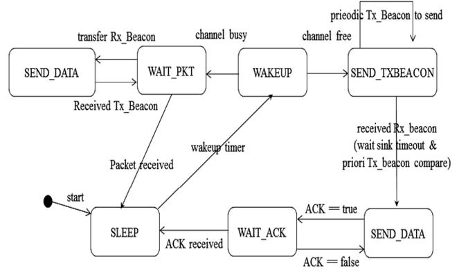
Fig. 9 Proposed mechanism MAC layer-finite state machine
