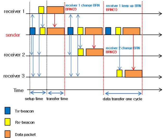
Fig. 3 receiver node efficient data packet transmission mechanism
