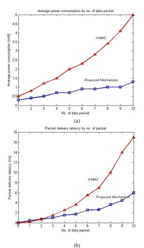
Fig. 10 Energy consumption & delay of 1-hop node from the sink. (a) average power consumption vs. no. of the packet (b) packet delivery latency vs. no. of the packet.
