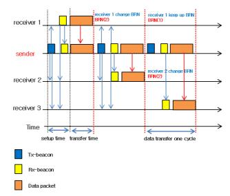
Fig. 3 receiver node efficient data packet transmission mechanism
