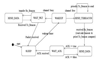
Fig. 9 Proposed mechanism MAC layer-finite state machine
