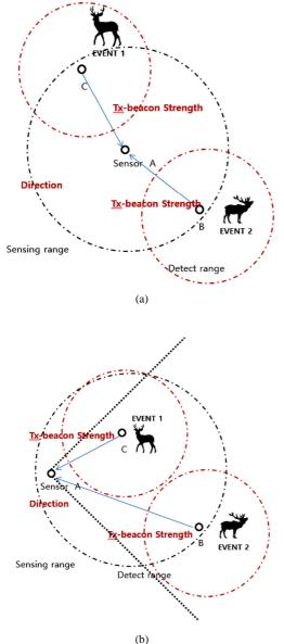
Fig. 7 Examples of duplicated packet decision error cases (a) by only strength (b) by the only direction
