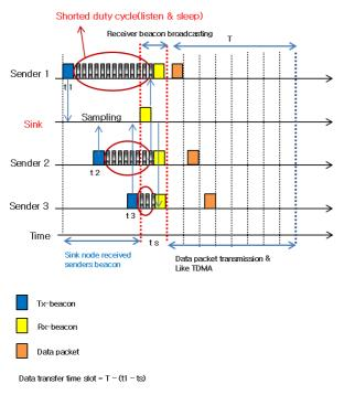
Fig. 5 Data transmission between a sink node and nodes.
