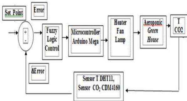
Fig. 1 Block diagram of temperature and CO<sub>2</sub> fuzzy control system on aeroponic greenhouse
