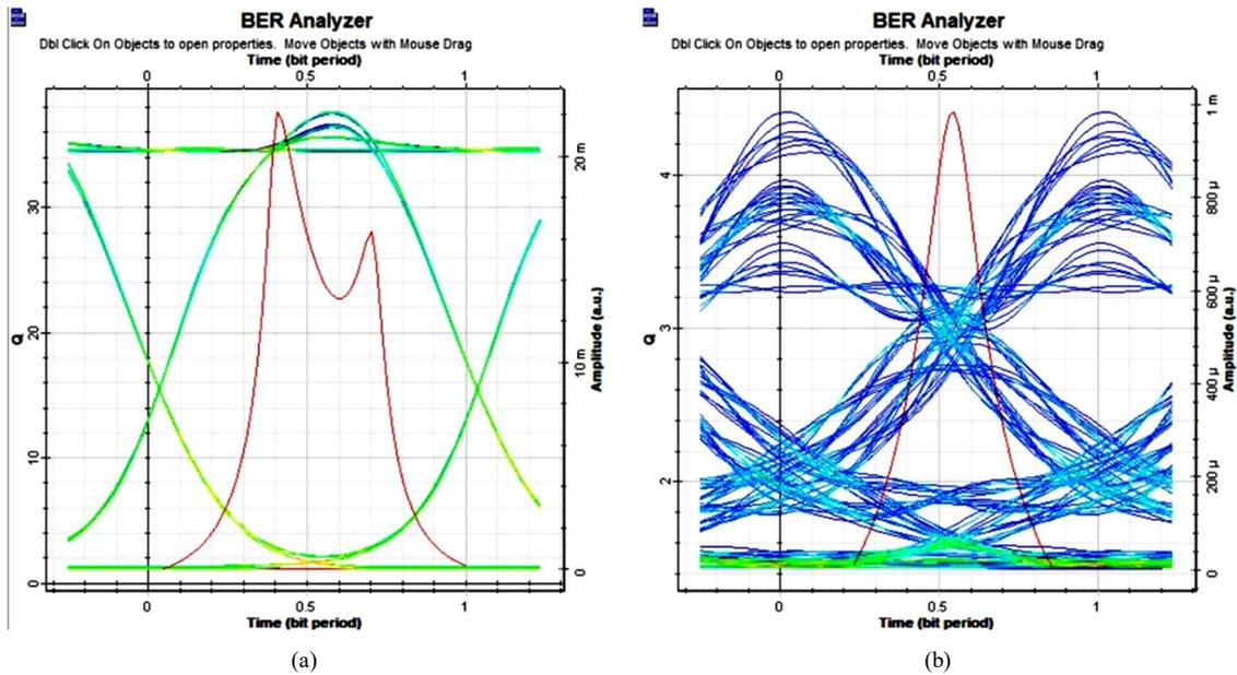
Fig. 7 Eye diagram of signal at input power of 10 dBm for (a) 10 and (b) 100 km
