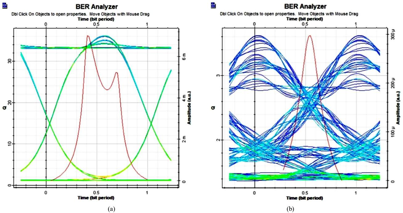
Fig. 6 Eye diagram of the signal at an input power of 5 dBm for (a) 10 and (b) 100 km
