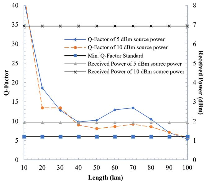
Fig. 4 Effect of GVD and SPM on Q-factor and received power
