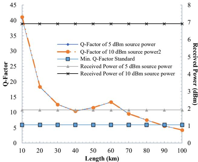
Fig. 3 Effect of GVD on Q-factor and received power
