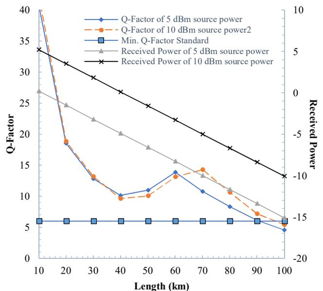
Fig. 5 Q-factor and received power for input powers of 5 and 10 dBm
