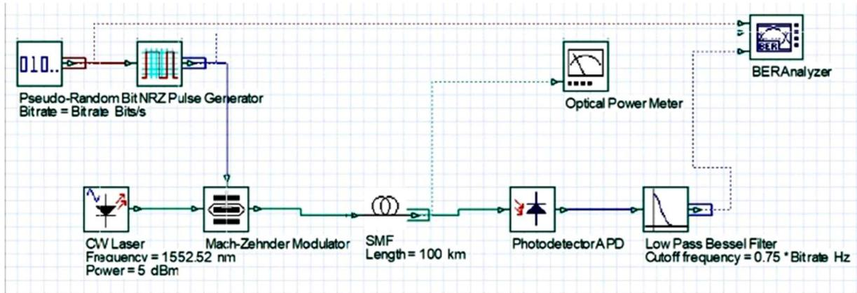
Fig. 1 Schematic of the optical fiber line system
