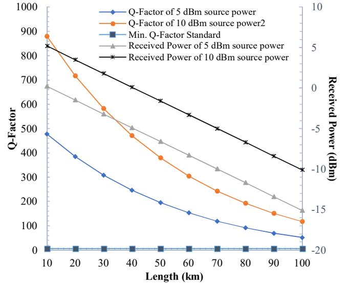
Fig. 2 Effect of attenuation on Q-factor and received power
