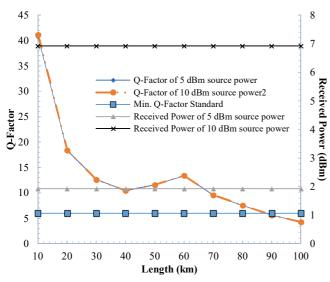
Fig. 3 Effect of GVD on Q-factor and received power
