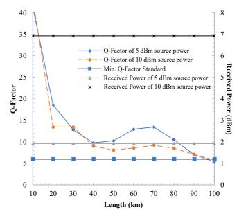
Fig. 4 Effect of GVD and SPM on Q-factor and received power
