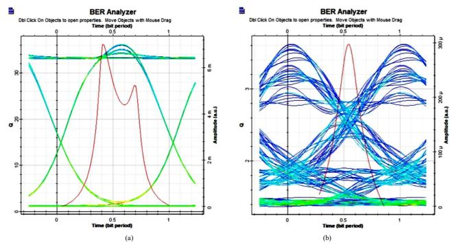
Fig. 6 Eye diagram of the signal at an input power of 5 dBm for (a) 10 and (b) 100 km
