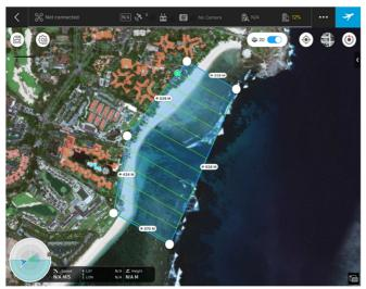
Fig. 6 Drone trajectory using the DJI GS Pro Software
