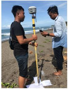
Fig. 7 Measurement of GCP coordinates
