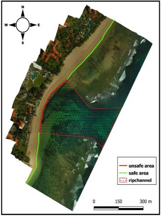
Fig. 12 Surf zone mapping from UAV-orthophoto.
