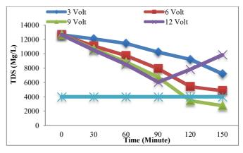
Fig. 5 The Effect of Electrocoagulation Process on TDS reduction
