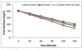
Fig. 17 The Effect of Electrocoagulation Process on Total hardness reduction
