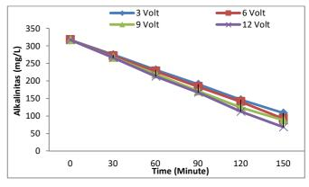
Fig. 14 The Effect of Electrocoagulation Process on Alkalinity reduction
