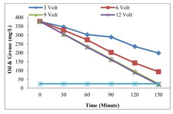
Fig. 11 The Effect of Electrocoagulation Process on oil & grease reduction
