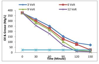
Fig. 13 Effect of Combination Process between Electrocoagulation and Adsorption on oil & grease reduction
