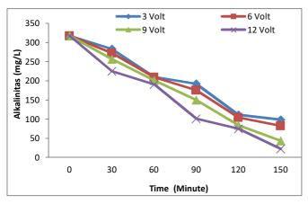
Fig. 16 Effect of Combination Process between Electrocoagulation and Adsorption on Alkalinity reduction
