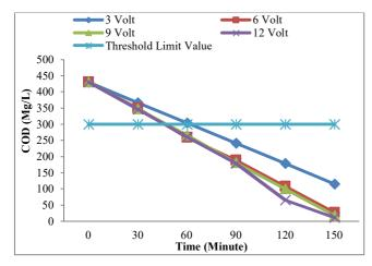
Fig. 4 Effect of Combination Process between Electrocoagulation and Adsorption on COD reduction
