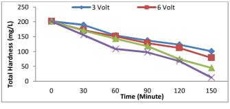
Fig. 19 Effect of Combination Process between Electrocoagulation and Adsorption on Total hardness reduction
