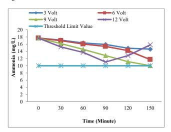
Fig. 8 The Effect of Electrocoagulation Process on Ammonia reduction
