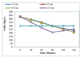
Fig. 2 The Effect of Electrocoagulation Process on COD reduction
