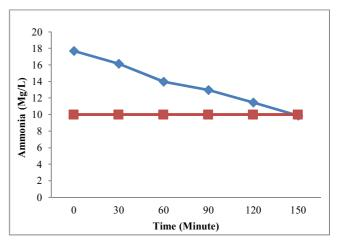
Fig. 9 Effect of the adsorption process on Ammonia reduction
