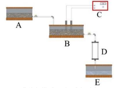
Fig. 1 Produced Water Treatment Process Equipment Design Note: A. Produced water storage tank; B. Electrocoagulation reactor; C. Power supply; D. Adsorption tube; E. Produced water treatment tank
