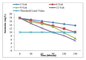
Fig. 10 Effect of Combination Process between Electrocoagulation and Adsorption on Ammonia reduction
