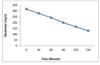
Fig. 15 Effect of the adsorption process on Alkalinity reduction
