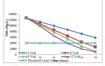
Fig. 7 Effect of Combination Process between Electrocoagulation and Adsorption on TDS reduction
