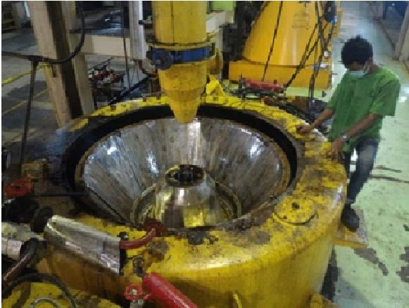
Fig. 1 Conical continuous centrifuges
