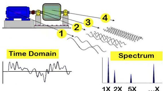
Fig. 2 Vibration frequency extraction
