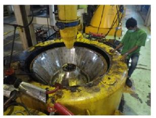
Fig. 1 Conical continuous centrifuges
