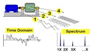
Fig. 2 Vibration frequency extraction
