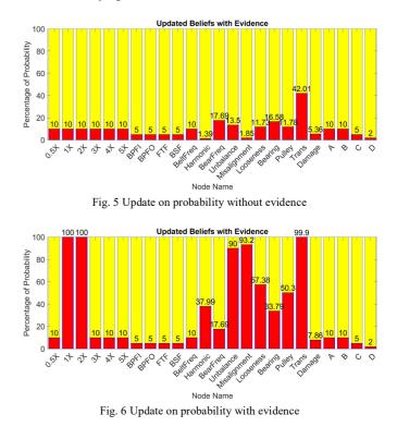
Without evidence of the probability, value of Unbalance was 13.5%; Misalignment 1.85%; Looseness 11.73%; Bearing 16.58%; Pulley 11.78%; and results in the probability of centrifugal damage was 5.36%. All probability values were still less than 50%; this indicated no damage to the centrifuges.
