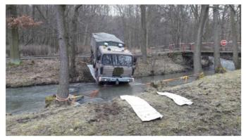
Fig. 3 Passes of the vehicle with plastic mats - both directions [25]
