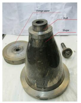
Fig. 4 Modified mandrel for the manufacture of carbon fiber billet
