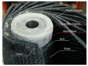
Fig. 6 Laying material packages on a mandrel
