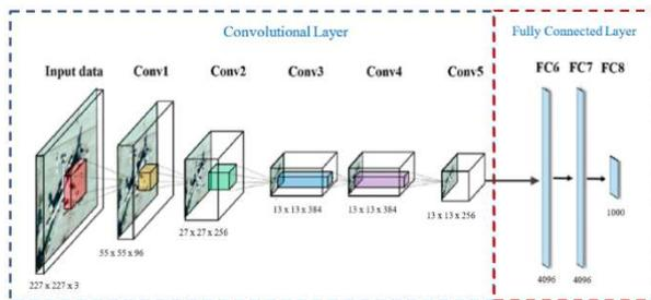
Fig. 3 AlexNet Architecture [14], [21]
