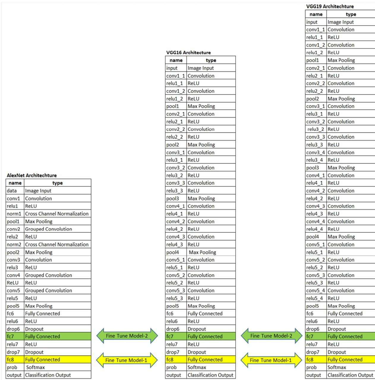
Fig. 5 Proposed fine-tuning on pre-trained network
