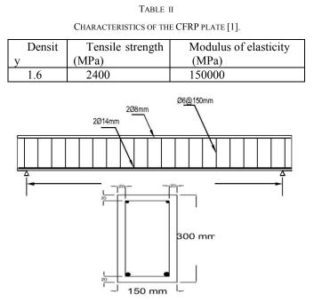
Figure (4): Beams dimensions and reinforcement details [1].
