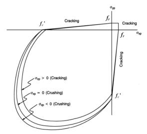
Figure(2)- 3D-failure surface for concrete [8].
