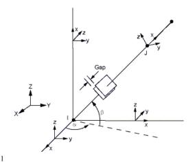
Figure (8) the contact element geometry (CONTAC52)[8].
