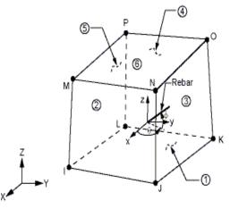
Figure (6): The solid element geometry (SOLID65)[8].
