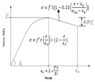
Figure(1): Uniaxial stress-strain of concrete in compression[7].
