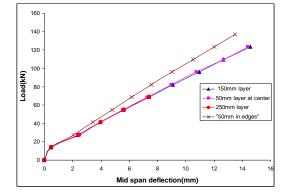
Fig.(12): The different locations CFRP beams load - deflection curve.
