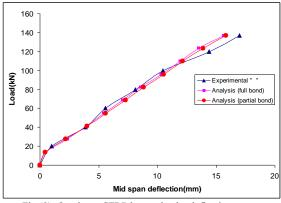
Fig.(9) :One layer CFRP beams load - deflection curve.
