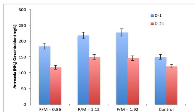
Fig. 6 The reduction of ammonia (NH<sub>3</sub>) concentration during the anaerobic decomposition
