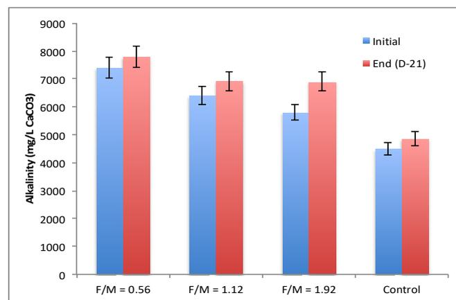
Fig. 5 The difference of alkalinity (as CaCO<sub>3</sub>) concentration at the initial and end of the experiment
