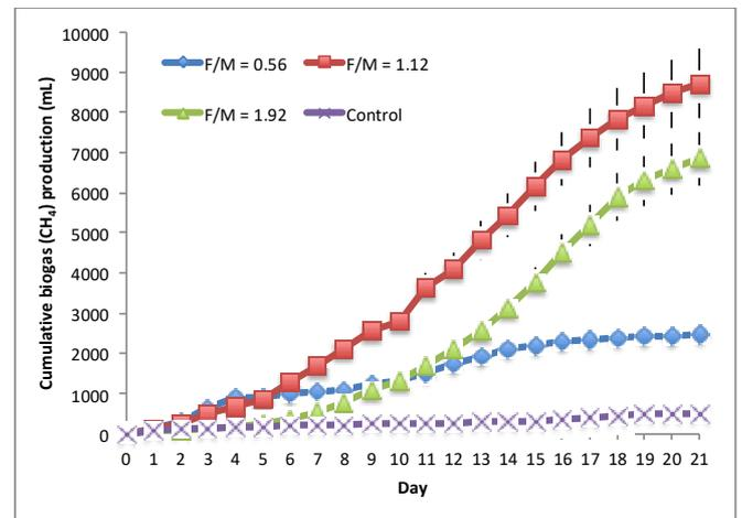
Fig. 2 Cumulative methane production from different F/M ratio
