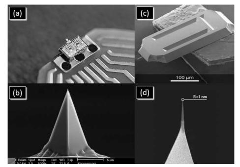
Fig. 4 Laser tip profile for high resolution and extra reinforcement hollow tube. (a). Single MEMS chip coarse apart augments sub-angstrom accuracy at lowest light leakage (b). Highly resonant, reflex coating compliments the plug and fit alignment (c). Tetrahedral tip at the end of the cantilever for correct ROI on the specimen (d). At the gold-coated silicon etched probe, resistive to reflectivity in the air well defined extra tip of carbon spike diamond.
