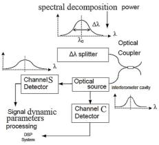
Fig. 3 Simplified view of ConLSCI sensor in Confocal
