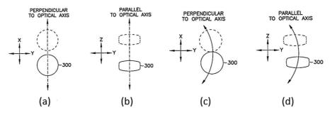
Fig. 5 Fabry-Prerot Cavity Impact on 3-D Coherence of Reference Channel. a), c) are orthogonal projection to illuminated axis, b), d) are Parallel to optical or illuminated axis.
