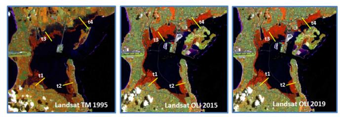
Fig. 3 The appearance of Mangroves using NIR + SWIR + Red composite bands and Spectral Transect Locations
