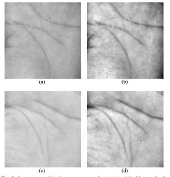
Fig. 5 Contrast stretching image preprocessing, (a, c) original image (b, d) contrast stretching image
