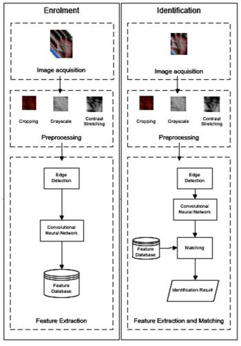
Fig. 2 Overview diagram of enrollment and identification process
