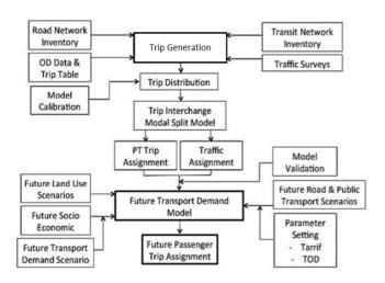
Fig. 4 Flowchart of the four-stage method (FSM)
