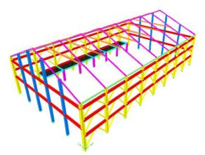
Fig. 5 The 3D model of the structure with steel bracing on X-direction
