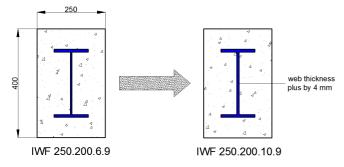
Fig. 8 The detail of adding the 4 mm of IWF web thickness (beam L=4.6 m)
