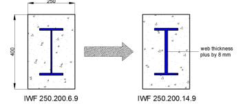
Fig. 9 The detail of adding the 8 mm of IWF web thickness (beam 4.25 m)
