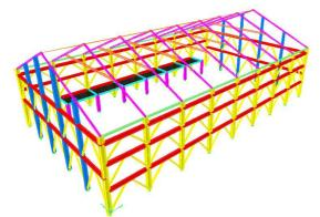
Fig. 7 The 3D model of the structure with steel bracing on X and Y-directions
