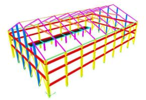
Fig. 6 The 3D model of the structure with steel bracing on Y-direction
