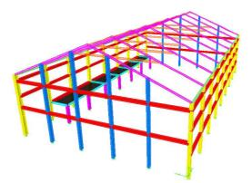
Fig. 3 The 3D modeling of the existing building
