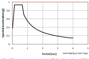
Fig. 4 The response spectrum design of Padang for medium soil [9]
