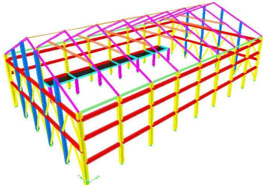
Fig. 6 The 3D model of the structure with steel bracing on Y-direction
