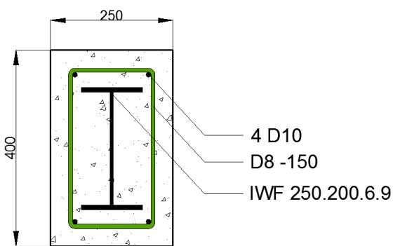
Fig. 10 The detail of strengthening by adding the reinforcement bars.
