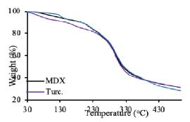
Fig. 1 TGA curve of of turmeric, maltodextrin and maltodextrin-ethanolic curcumin extract
