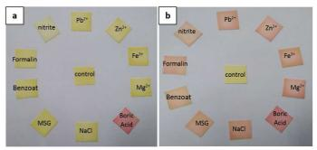
Fig. 7 Detection of curcumin paper strip towards 10000 ppm of various sole chemicals (a), chemicals + boric acid mixture (b).
