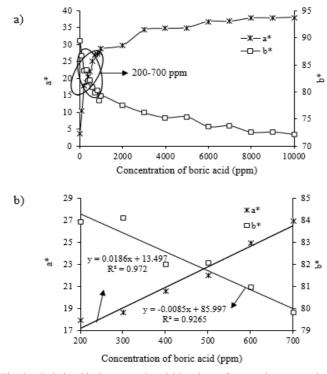
Fig. 9 Relationship between  $a^*$  and  $b^*$  values of curcumin paper stripboric acid and concentration of boric acid from 100 to 10000 ppm (a) calibration line drawn for boric acid sensing by curcumin paper strip based on  $a^*$  and  $b^*$  (b)
