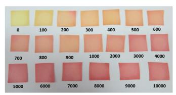
Fig. 8 Color scale of the curcumin paper strip response to various concentration of boric acid solution from 100-10000 ppm
