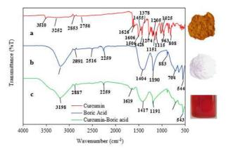
Fig. 3 FTIR spectra of curcumin (a), boric acid (b), and curcumin-boric acid (c)
