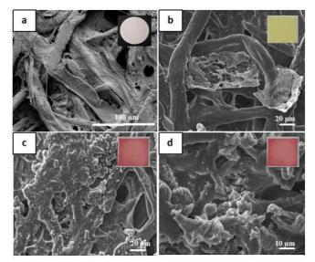
Fig. 6 SEM images of filter paper (a), curcumin paper strip surface (b), curcumin paper strip-boric acid surface (c) curcumin paper strip-boric acid, cross section (d)
