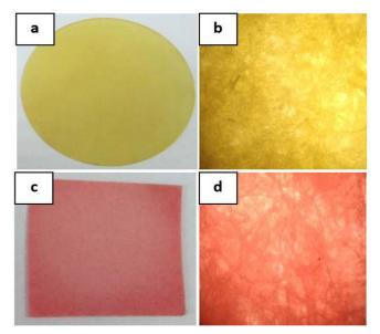
Fig. 5 Appearance of curcumin paper strip (a), optical microscope image of curcumin paper strip (b), curcumin paper strip upon contact with boric acid (c), optical microscope image of curcumin strip-boric acid (d)
