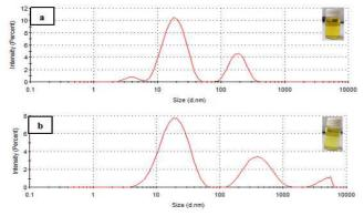
Fig. 2 Curve of particle size distribution for CURNns (a), and CURNnsr (b)
