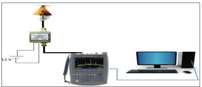
Fig. 3 The RFI connection setup
