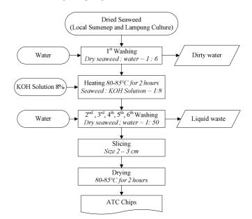
Fig. 2 Flow diagram of processing ATC
