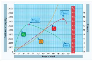
Fig. 3 Aircraft performance versus angle of attack [18].
