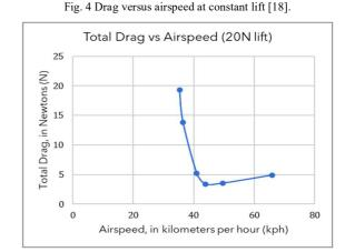
Fig. 5 Total drag versus airspeed of the fixed-wing drone at 20N of lift.
