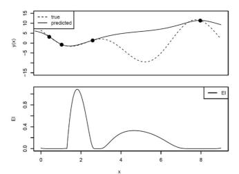
Fig. 7 Optimization using Gaussian process in the EGO framework [20].
