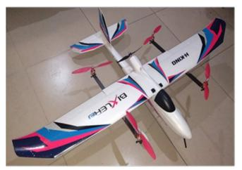
Fig. 1 Separate-lift-and-thrust hybrid drone
