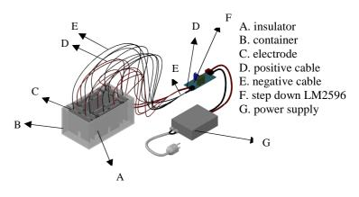
Fig. 1. Electrocoagulation design
