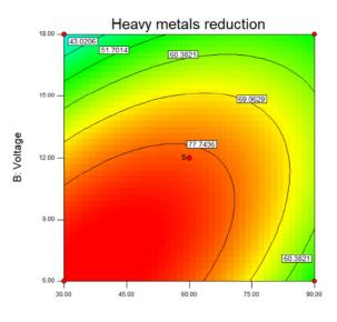
A: Immersion time Fig. 3. Contour plot of heavy metals reduction
