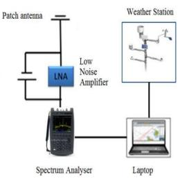
Fig. 3 Receiver system setup [15], [16], [17]
