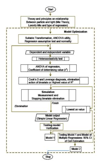
Fig. 2 Algorithm of obtaining and testing models; model 1 is a turbidity standard curve; model 2 is multiple regressions for the medium of multiplied cell. The optimal workflow has been structured
