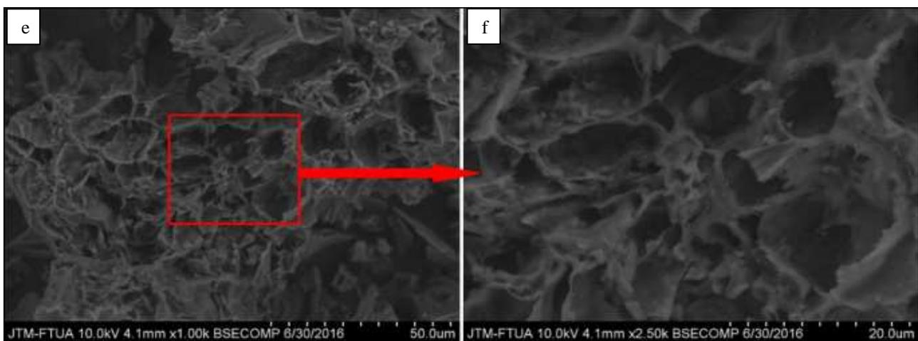
Fig. 9 SEM photos adsorbent with activator ACHJ at HCl 0.1 M. (e) magnification 1000x (f) magnification 2500x
