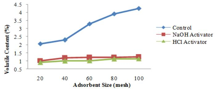
Fig. 3 Effect of size and type activators adsorbent against volatile content on adsorbent ACHJ
