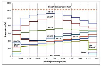
Fig. 7 The temperature of the pebble in the core, graphite and carbon brick reflector, reactor internal space, vessel, and air in the RCCS cavity
