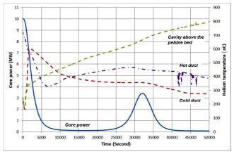
Fig. 5 Transients of the core power and helium temperature in the primary system
