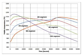
Fig. 6 Transient of pebble temperature (5 lowest segments) in the middle core following the event with the insertion of FTC
