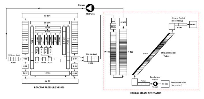
Fig. 3 The integrated model of RDE Nuclear Steam Supply System (NSSS) developed by RELAP5 code
