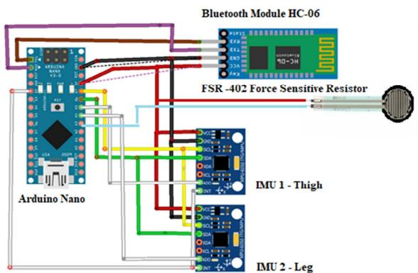
Fig. 3 The electronic scheme of the prototype developed to capture the measurements.
