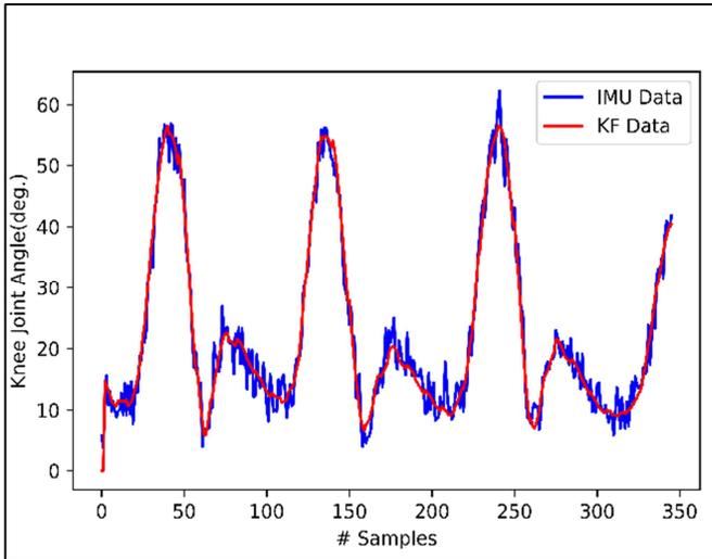
Fig. 6. Kalman Filter and Knee Angle Estimation Model
