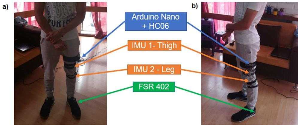
Fig. 2 Subject wearing develop system with IMU sensors: a) subject in front view; b) subject in sagittal view.
