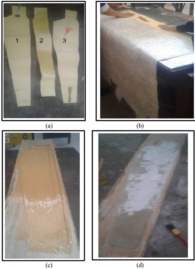
Fig. 3 The manufacturing of blade. (a) the fiberglass mat shape, (b) chopped strand fiberglass mat, (c) blade mold, (d) fiberglass molding process
