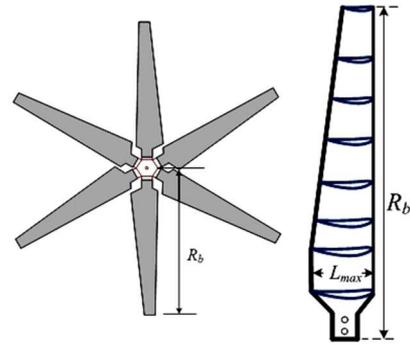
Fig. 1 Design of HAWT blade
